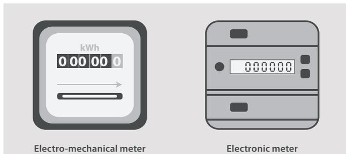
**An electro-mechanical meter** is a meter fitted with one or several numbered dials which are rotated by a metal disc.
