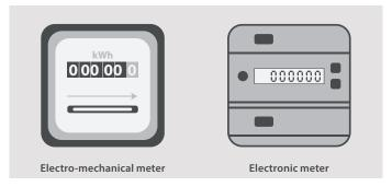
An electro-mechanical meter is a meter fitted with one or several numbered dials which are rotated by a metal disc.
